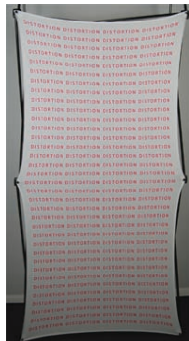
1" in - distortion very noticeable
