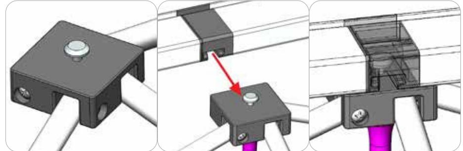
The scissor frames will have middle hubs with a metal prong installed on all four sides front and left and right sides of back. Attach the middle caps of the channel bars onto the middle hubs. The middle caps of the channel bar will snap into place.
