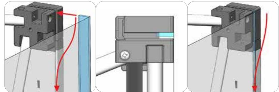
As an optional feature, the front printed graphic may have end cap graphics with silicone edge. Pull the end cap silicone edge to the top of the back corner hub. Start to press in the SEG into the hub and work your way down the side channel. Do the same for the opposite end cap.
