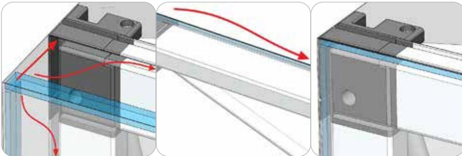
To apply the silicone edge graphic, start by pressing the SEG into the top left corner hub of the frame. Continue to press the SEG into the extrusion bar fabric channel. Keep pressing the SEG into the bar fabric channel until you make down to the bottom right corner hub of the frame. This also works for the second printed graphic option on the back side of the frame when horizontal channel bars are installed.
