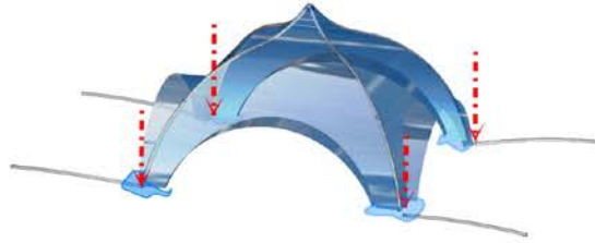
1- ALIGN AND CENTER FABRIC GRAPHIC WITH THE FRAME.
